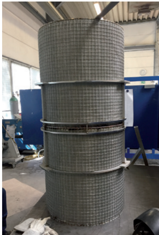
Figure 3: Completely new construction of a seawater filter element; materials from FIL-TEC RIXEN GmbH®
